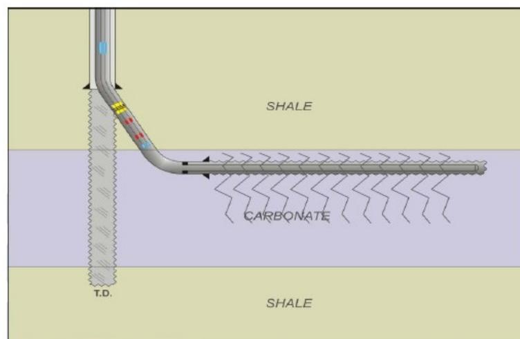
Figure 4: HW3 well drilling concept
